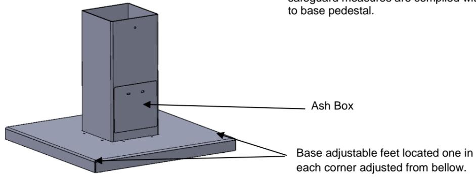
Lift and locate the fire body on to the base post. Note the fire body is a heavy item and should be lifted into position by two people. When in position secure in place with M6 fixing screw. Note the orientation of the fire body, the screw in the top corner of the top plate should be in the front left hand corner. This will mean that the fire door and the ash pan are on the same side.
