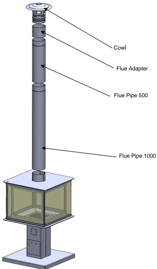
Fit Flue pipe sections and flue cowl as shown these are a push fit.
